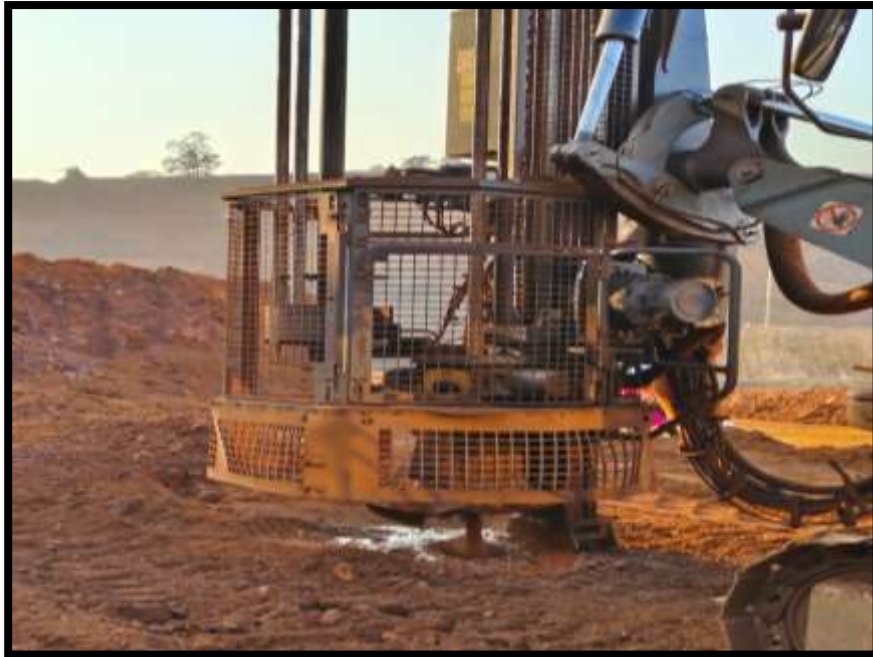
Wet Drilling System in Drilling Operation
